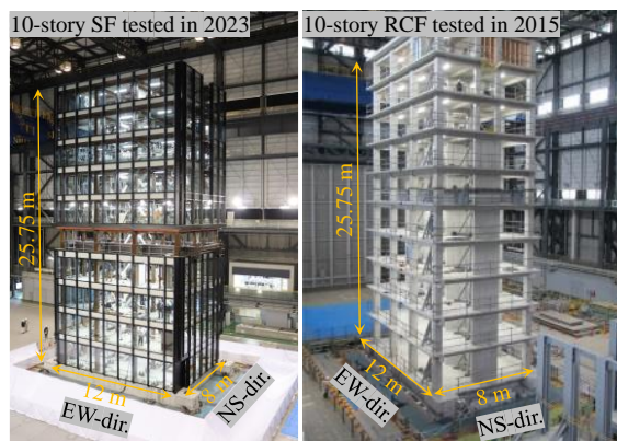
Fig. 1 10-story steel specimen and 10-story RC specimen
